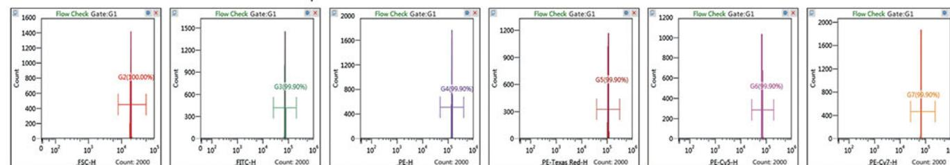
Excellent fluorescence detection limit: FITC < 50MESF, PE < 30MESF
